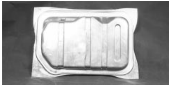
Fig. 14 Photographs of experimental specimens by a fuel tank deep drawing. (a) View-1. (b) View-2
